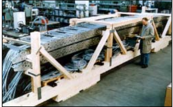
Varittrak S® - Open Style Super Duty Steel Carrier - Bored Aluminum Bars Dual Carrier Nested Carrier for Horizontal Operation - Sold and Delivered with Cables and Hoses Installed - Turn Key.
