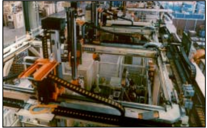
Plastitrak® - Open Style Nylon Carrier - Hinged Opening Bars Vertical & Horizontal - Operation in a Support Tray
