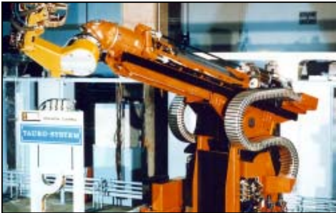
Conduflex® - Enclosed Stainless-Steel Tube Carrier Up & Down plus In & Out Operating Mode Robotics in Automotive Assembly
