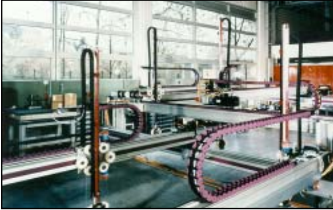
Varitrak ME® - Small Open Style Modular Nylon Carrier - Nylon Bars Vertical - Loop Up plus Horizontal Operating Modes Automation - Pick & Place Robots
