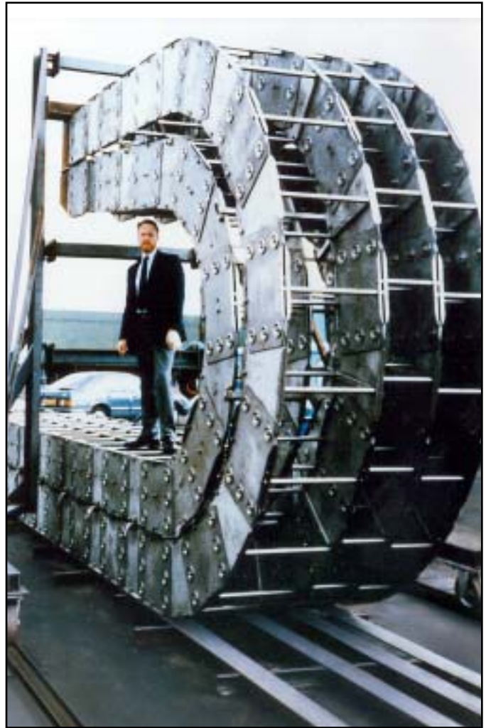
Varitrak S® - Open Style Super Duty Steel Carrier - Steel Rods with Delrin® Rollers and Rolling Dividers
