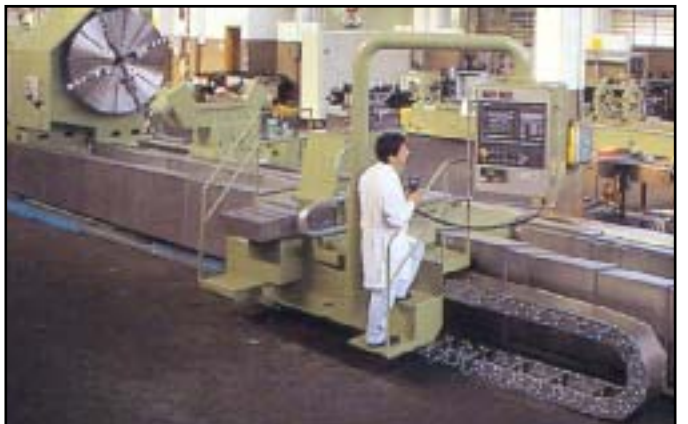
Varitrak S® - Enclosed Style Heavy Duty Steel Carrier with Stainless Steel Hot Chip Covers
