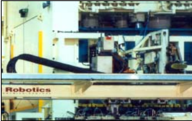
Varitrak MK® - Open Style Modular Nylon Carrier - Nylon Bars Horizontal Operating Mode in a Guide Channel
