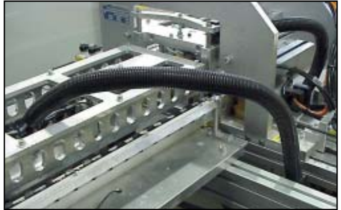
KabelFlex® - Highly Flexible Nylon Conduit Multi-Directional Horizontal Operation -Unsupported Automated Machinery
