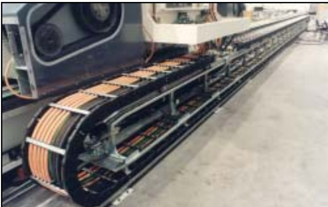
Varitrak MC® - Open Style Heavy Duty Nylon Carrier - Aluminum Bars Extended Horizontal Travel Operation with Moving Support Carriage. Automated Cutting
