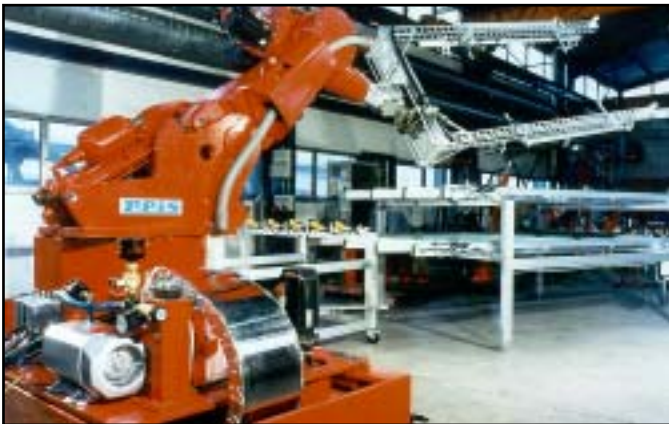
Varittrak S® - Enclosed Style Steel Carrier with Stainless Steel Hot Chip Covers
