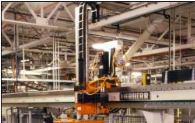
Varitrak MC® - Open Style Modular Nylon Carrier - Aluminum Bars Vertical - Loop Up plus Horizontal Operating Mode in a Guide Channel Automated Process Material Handling
