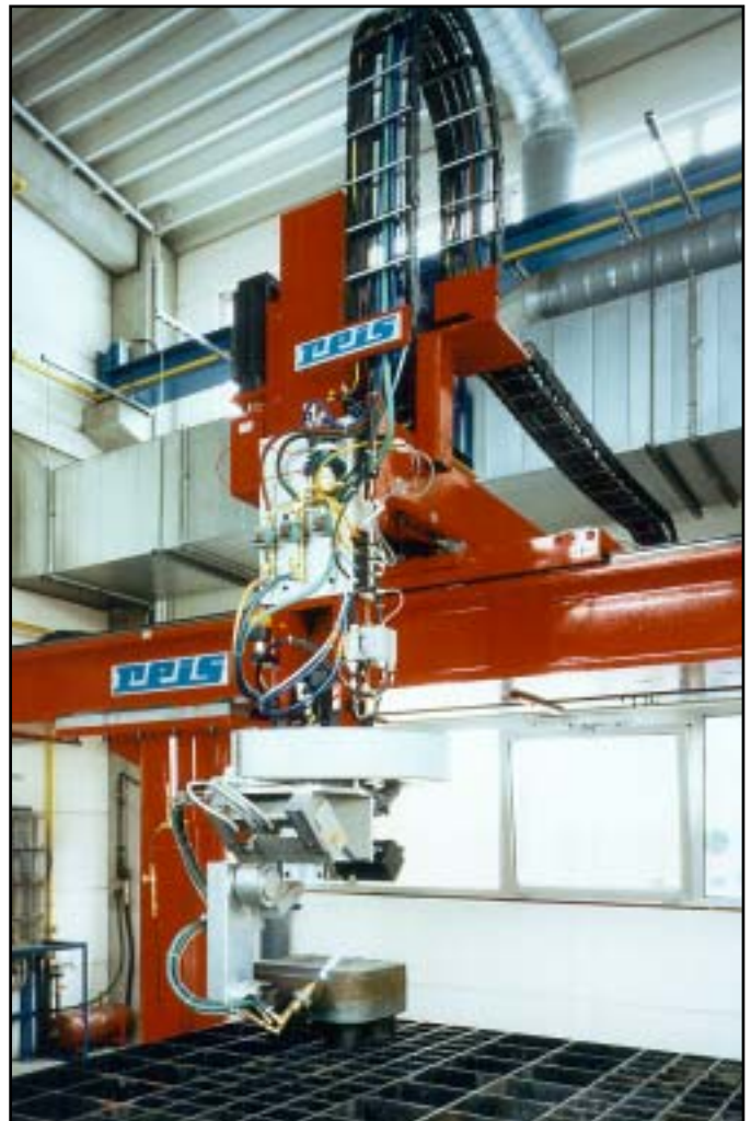
Varitrak K® - Open Style Heavy Duty Nylon Carrier - Aluminum Bars Vertical - Loop Up plus Horizontal Operating Mode
