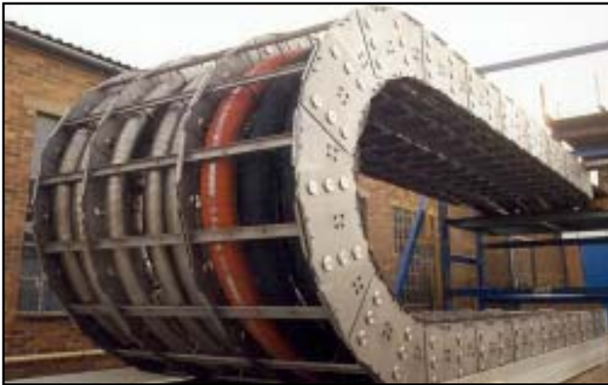
Varitrak S® - Open Style Super Duty Stainless Steel Carrier - Steel Bars Horizontal Operating Mode - Quad Band. Carrier sold and delivered with special hoses installed at KS Factory - Turn Key.
