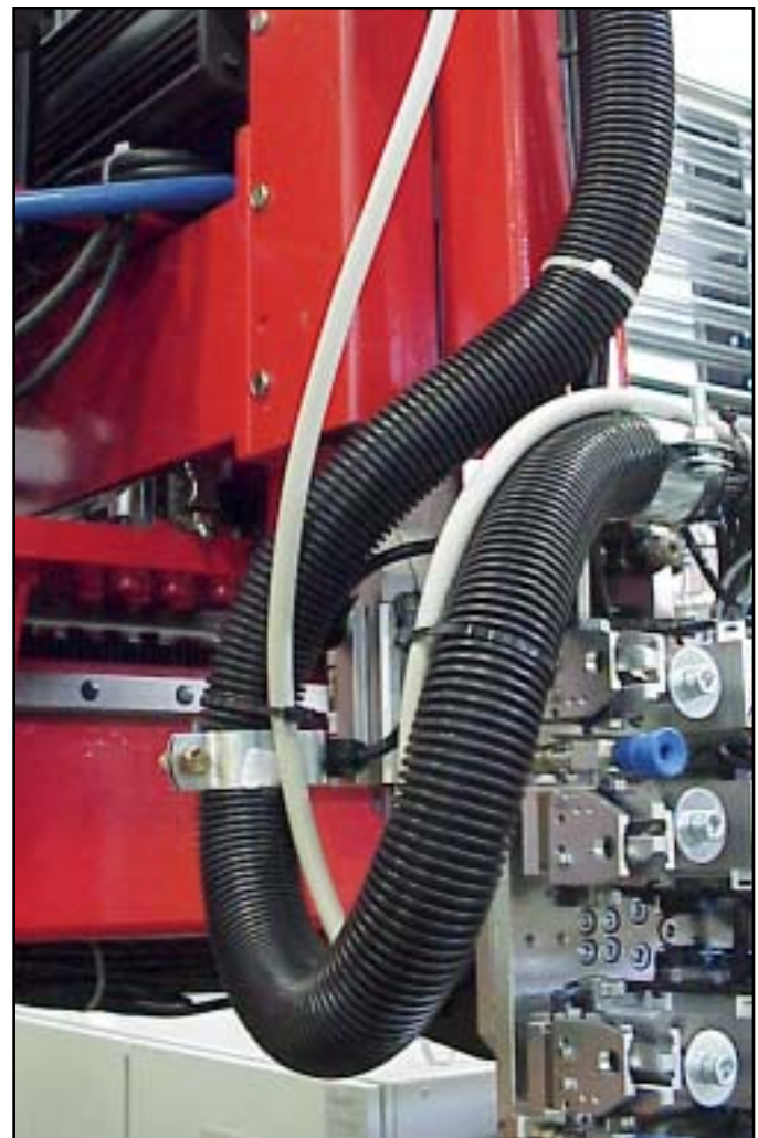
KabelFlex® - Highly Flexible Nylon Conduit Multi-Directional and Rotating Operation Automated Machinery
