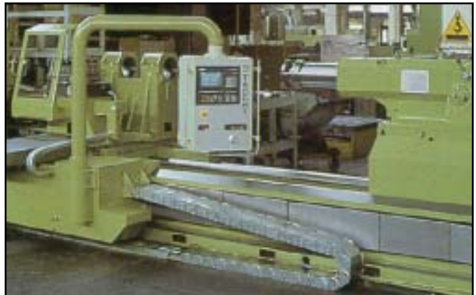
Varitrak S® - Enclosed Style Steel Carrier - Stainless Steel Hot Chip Covers
