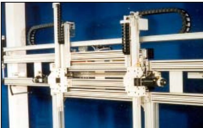
Plastitrak® - Open Style Nylon Carrier - Hinged Opening Bars Vertical - Loop Down plus Horizontal in Support Tray Operating Modes
