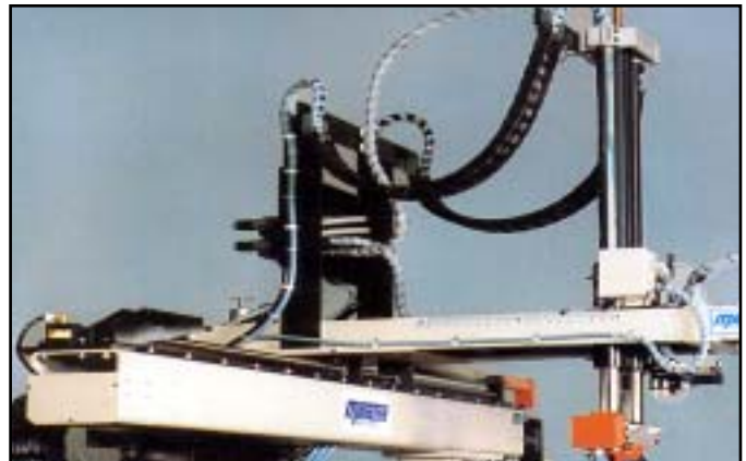
Versatrax® - Open Style Heavy Duty Nylon Carrier with Hinged Opening Bars Vertical - Loop Down/Hanging plus Horizontal Operating Modes Factory Automation
