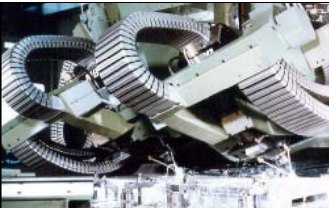
Conduflex® - Enclosed Stainless-Steel Tube Carrier X, Y and Z Axis Operating Modes Machine Tool
