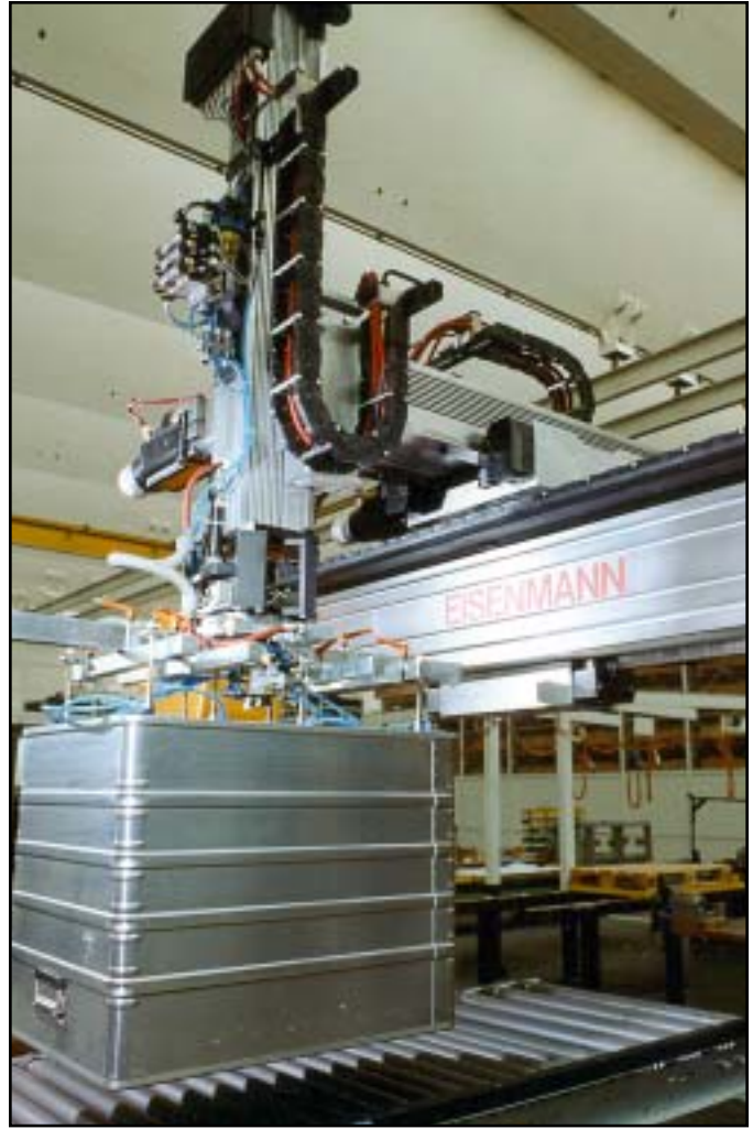
Varitrak K® - Open Style Heavy Duty Nylon Carrier - Aluminum Bars Vertical - Loop Down plus Horizontal Operating Mode Automated Process Material Handling
