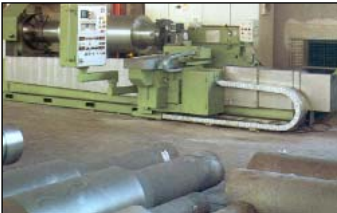
Varitrak S® - Tube Style Steel Carrier - Aluminum Bolted on Lids Horizontal Operating Mode with Support Braces
