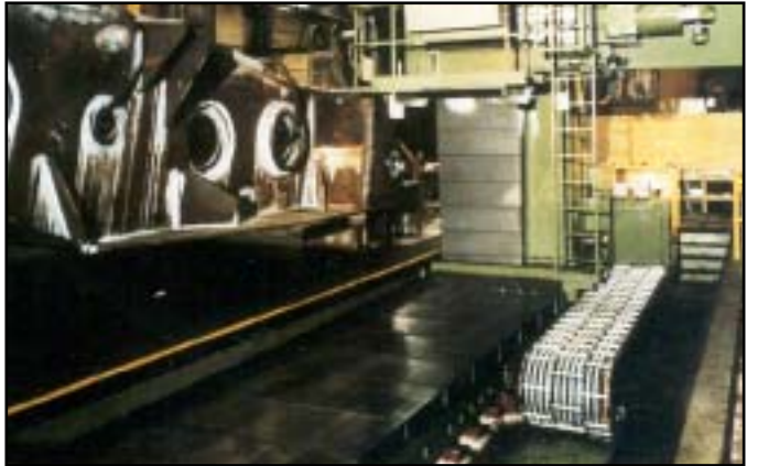
Varitrak K® - Open Style Heavy Duty Nylon Carrier - Aluminum Bars
