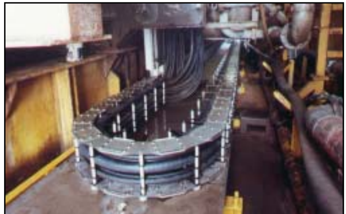
Varittrak S® - Open Style Heavy Duty Steel Carrier with Special Glide Pads Side Mount Operating Mode (to reduce vertical mounting height ) Processing Plant
