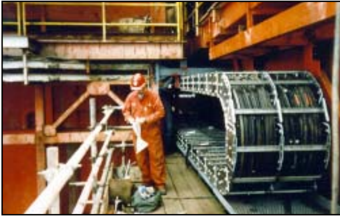
Varitrak S® - Open Style Super Duty Steel Carrier - Heavy Duty Steel Bars with Rolling Dividers
