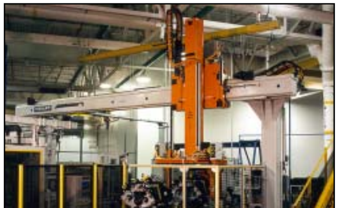
Varitrak K® - Open Style Heavy Duty Nylon Carrier - Aluminum Bars Vertical - Loop Up plus Horizontal Operating Mode in a Guide Channel Automated Process Material Handling
