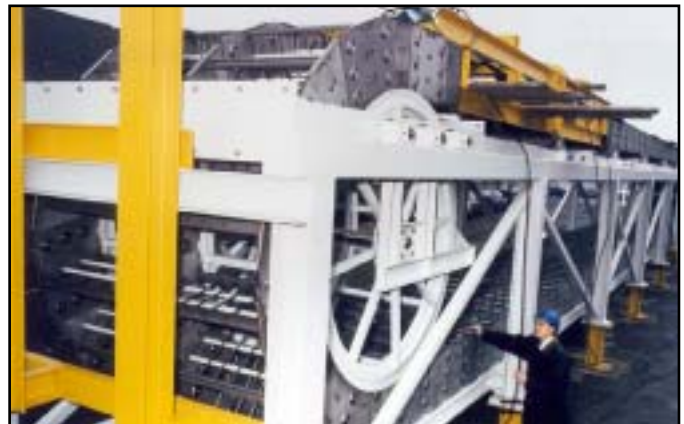
Varitrak S® - Triple Band Open Style Super Duty Stainless Steel Carrier - Steel Bars with Rolling Dividers
