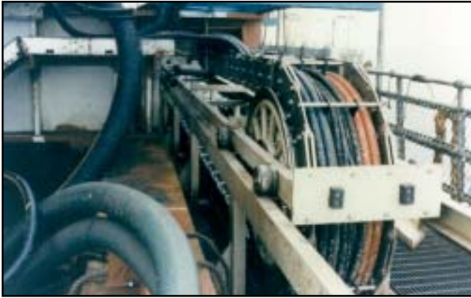
Varitrak S® - Open Style Super Duty Stainless Steel Carrier - Steel Rods with Delrin® Rollers and Nylon Dividers
