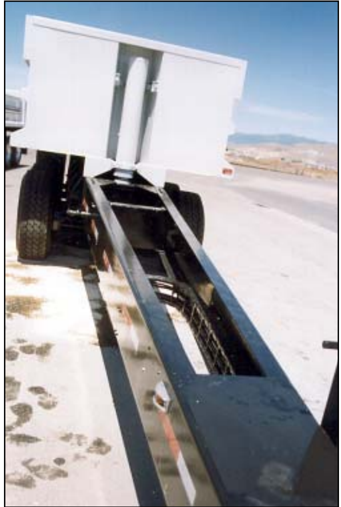
Varitrak K® - Open Style Heavy Duty Nylon Carrier - Aluminum Bars High Vibration Loads in a Horizontal Side Mount Operation Automatic Truck Trailer Hitch Spacing
