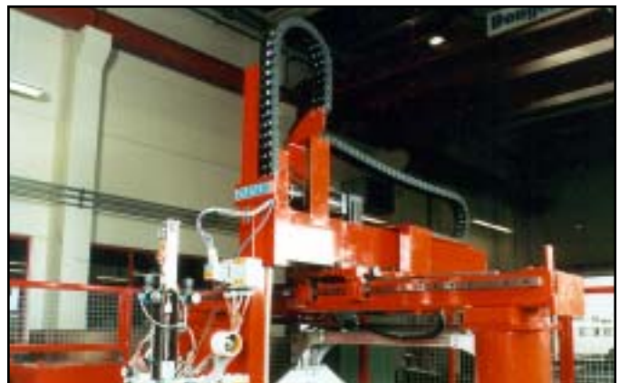
Plastitrak® - Open Style Nylon Carrier - Hinged Opening Bars Vertical - Loop Up plus Horizontal in Support Tray
