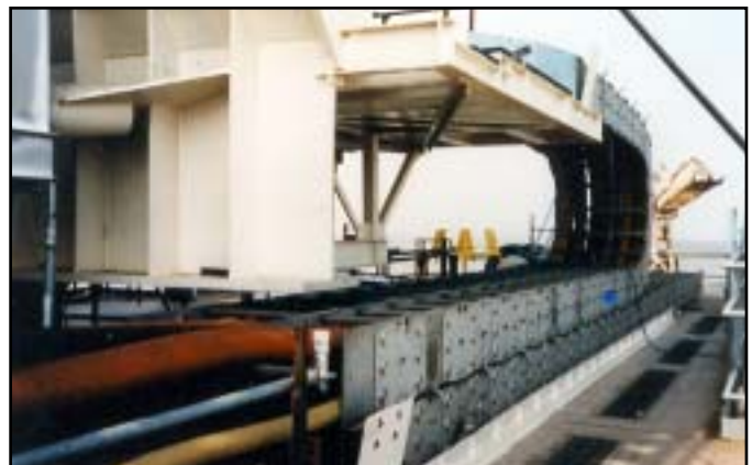
Varitrak S® - Nested Open Style Super Duty Steel Carrier - Steel Bars -Triple Band Construction.
