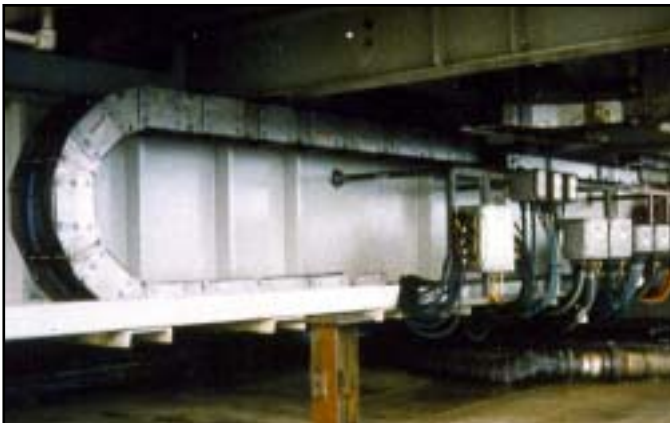
Varitrak S® - Open Style Super Duty Steel Carrier - Steel Rods with Rollers
