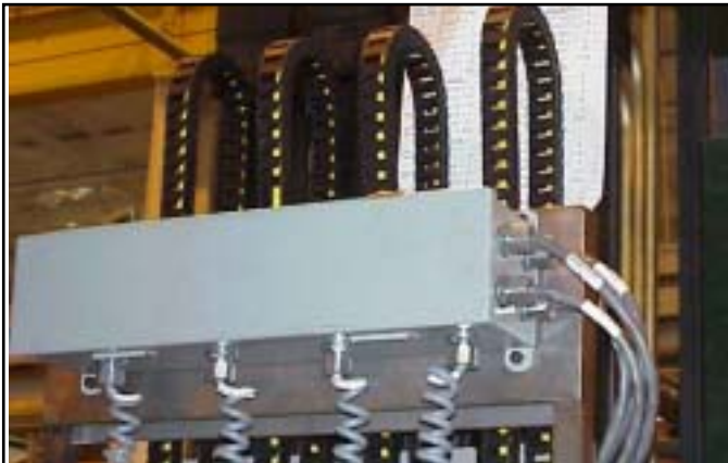
Microtrak® - Miniature Nylon Carrier - Hinged Opening Lids Horizontal Operating Mode Automated Process Equipment
