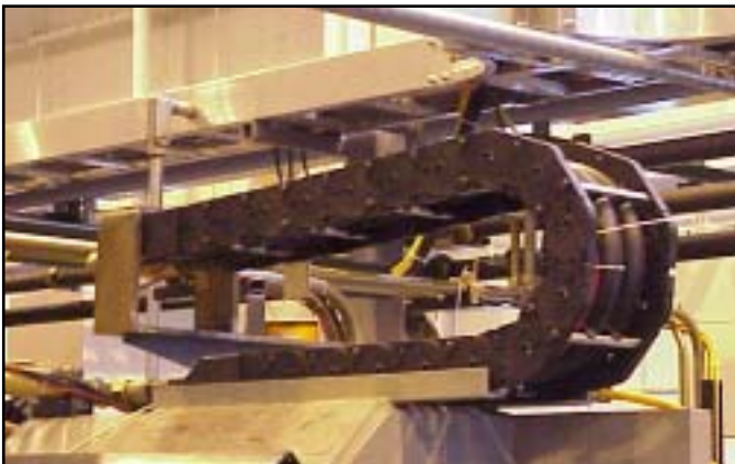
Varittrak K® - Open Style Heavy Duty Nylon Carrier - Aluminum Bars Horizontal Operating Mode Machine Tool
