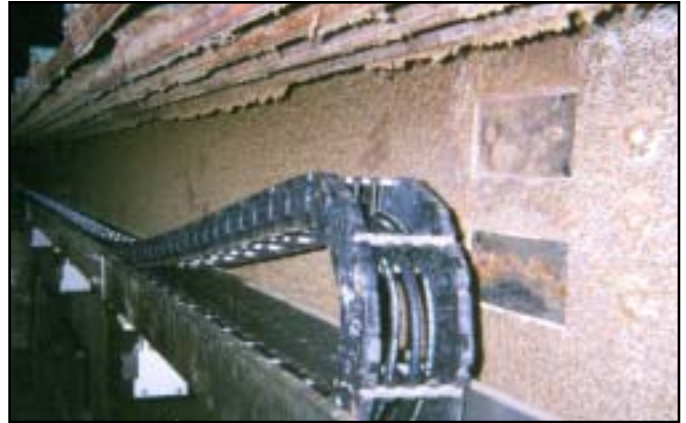
Varitrak MC® - Open Style Heavy Duty Nylon Carrier - Aluminum Bars Extended Horizontal Operating Mode in a Guide Channel
