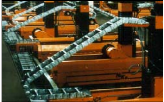
Varitrak S® - Open Style Steel Carrier - Aluminum Bars Horizontal and Vertical Operating Modes
