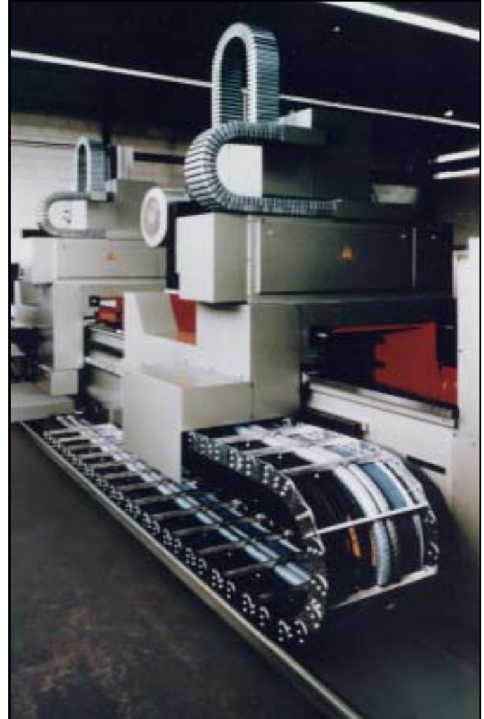
Varitrac S® - Open Style Steel Carrier - Bored Aluminum Bars
