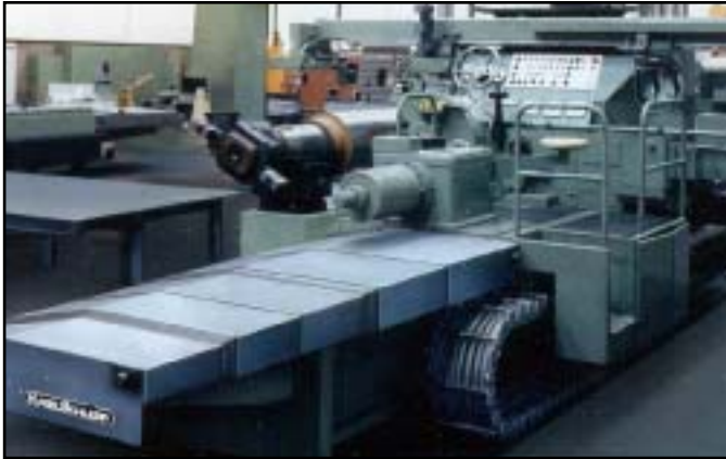
Varitrak S® -Open Style Steel Carrier - Bored Aluminum Bars Horizontal Operating Mode in a Support Tray
