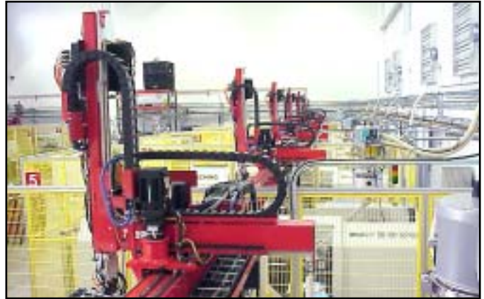
Varitrak K® - Open Style Heavy Duty Nylon Carrier - Aluminum Bars Horizontal Operating Mode in a Support Tray
