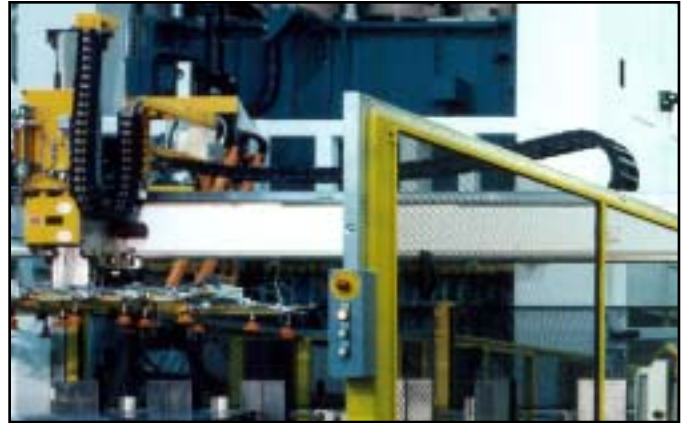
Varitrak MK® - Open Style Modular Nylon Carrier - Nylon Bars Vertical - Loop Down & Horizontal Operating Mode in a Guide Channel
