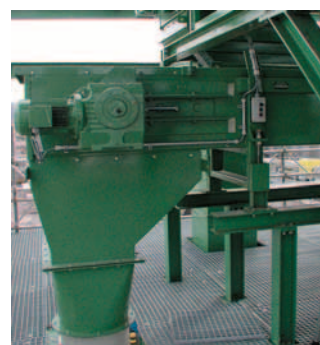
■ Scraper conveyor for distribution of various chip materials
