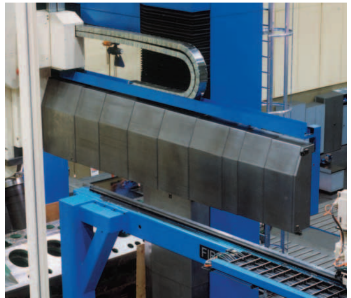
■ Cross-beam cover at a milling machine
