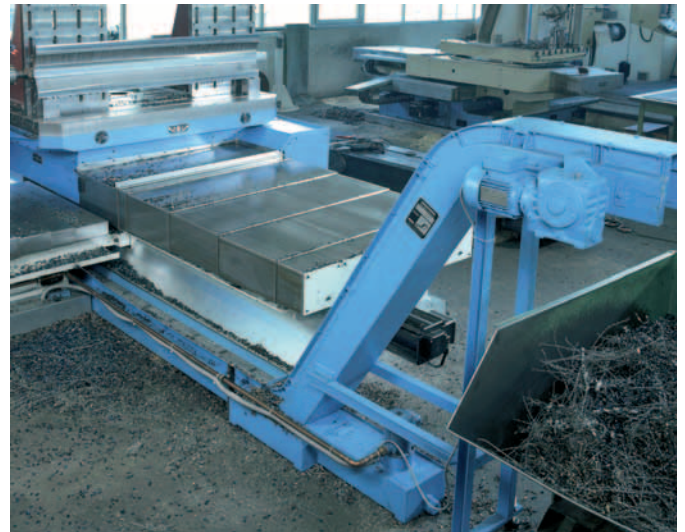
■ Standard hinged belt conveyor at a CNC boring machine
