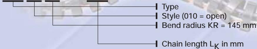
The correct order number for a completely assembled ROBOTRAX cable carrier system is composed of type, style, KR as well as carrier length. At present the open style 010 is available.
