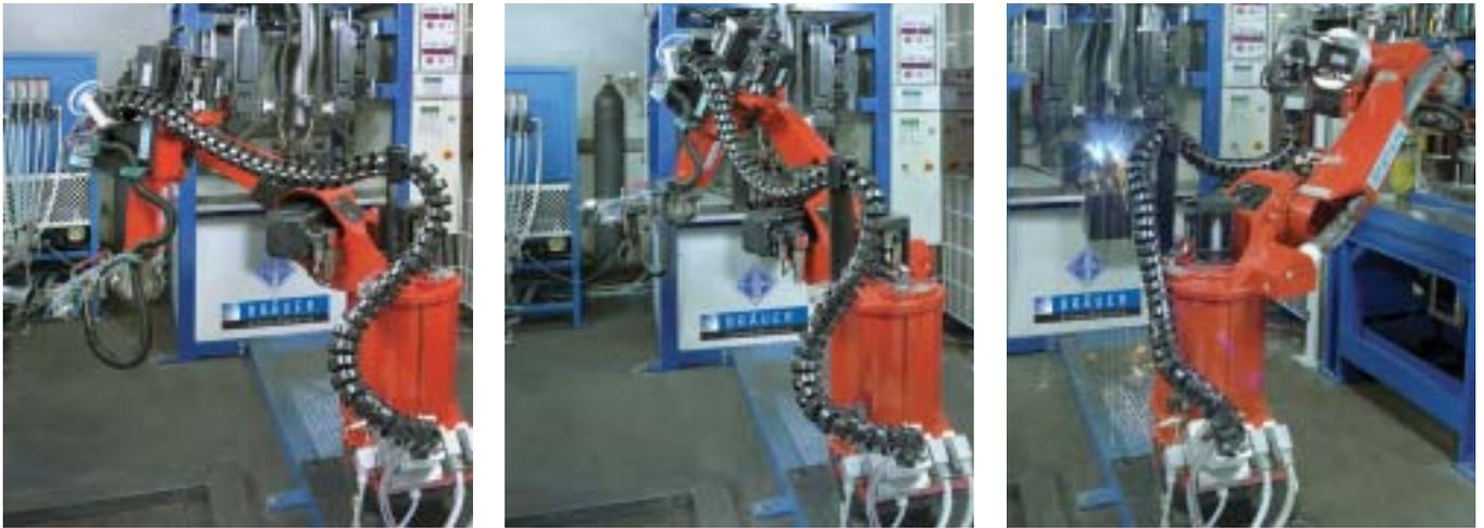
Rotation angle of approximately 180° without a guide channel on an articulating arm robot application
