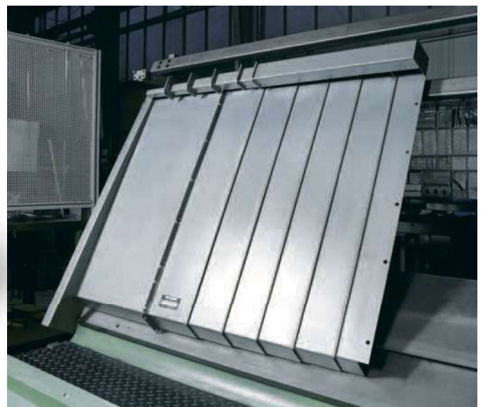
■ Special form of an inclined bed cover on a test framework
